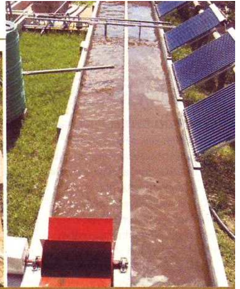
ABOVE, LEFT TO RIGHT: Views of the pilot plant's 20m 2 raceways, where algae is farmed. The algae is initially sourced from the farm's dam. They then anaerobically digest stillage containing residual cellulose, starch and proteins. The solar panels are used to power the system. The end product is a bucket of green algae, harvested for conversion into bioethanol. PHOTOS: REX ZIETSMAN
